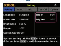
When multiple power supplies are in serial or parallel connection, enabling the external trigger function can realize the synchronous output for multiple power supplies.
