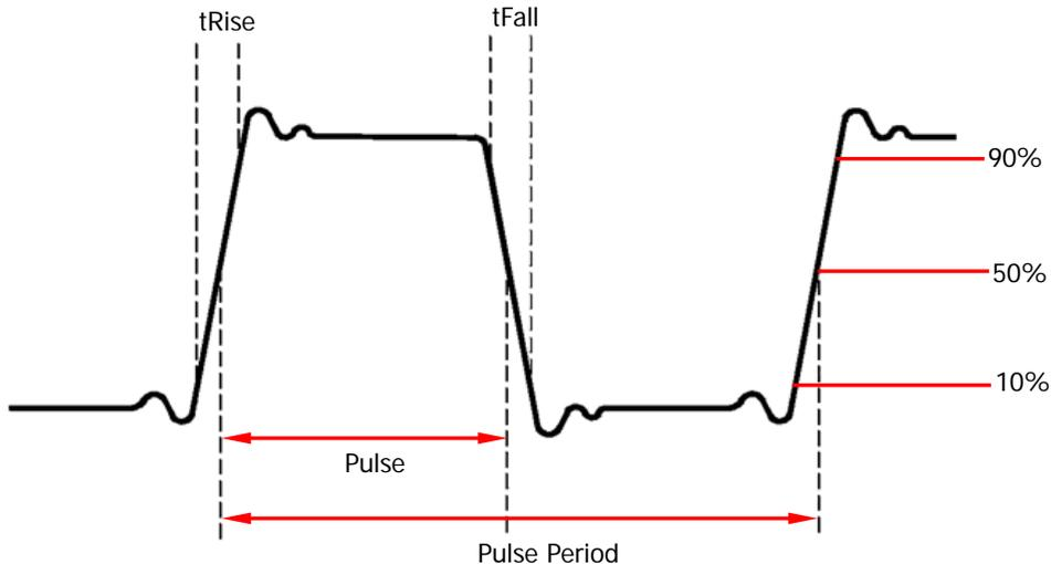
The settable range of the pulse width is from 16 ns to 999.999982118 ks (limited by "minimum pulse width" and "pulse period"). The default is 500  $\mu$ s.
