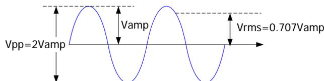
According to the figure above, the conversion relation between  $V_{pp}$  and  $V_{rms}$  fulfills the following equation:
