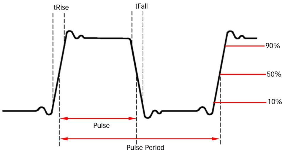
Tap the **RisEdge** or **FallEdge** parameter input field. Use the numeric keypad to input the desired value and then select the desired unit from the pop-up menu.
