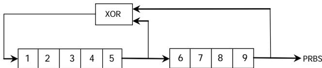
An LFSR is specified by the number of stages it contains ( $L$ ) and which stages (taps) feed the exclusive-or (XOR) gates in its feedback network. The PRBS output is taken from the last stage. After selecting proper taps, an  $L$ -stage LFSR produces a repetitive PRBS of length  $2^L - 1$ . The clock frequency of LFSR determines the "bit rate" of PRBS.
