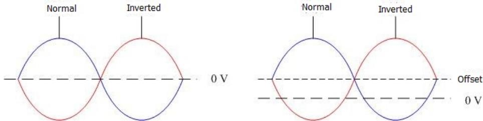
**Note:** When the waveform is inverted, the sync signal related to the waveform is not inverted. To set the invert of the sync signal, tap **SyncSet** → **Polarity** to select "Negative".
