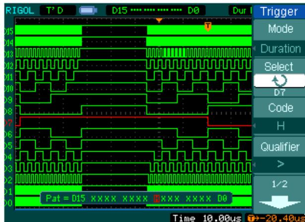
Figure 3- 13 Duration Trigger on a digital signal
