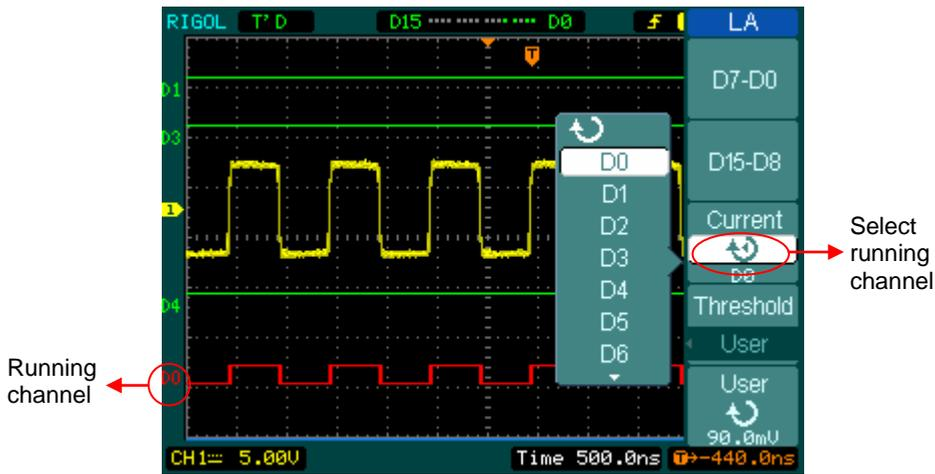
Figure 2- 32 Turn on the digital channel
