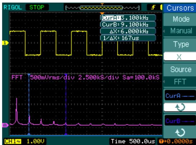
Figure 3- 10 The example of Cursor measuring FFT frequency
