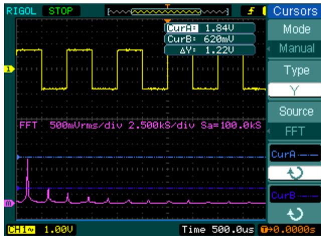
Figure 3- 9 The example of Cursor measuring FFT amplitude
