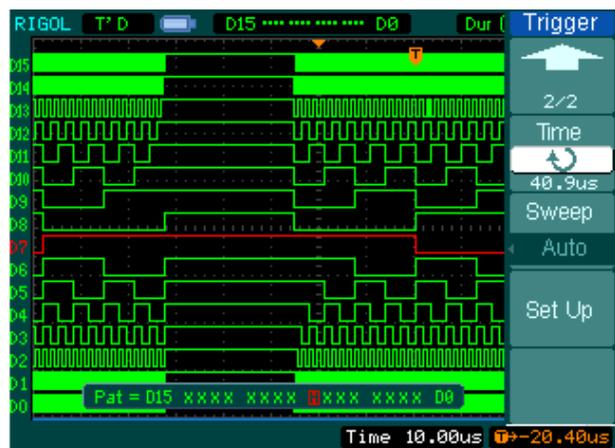
Figure 3- 14 Duration Trigger on a digital signal
