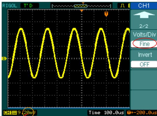
Fine adjustment data Figure 2- 12 Fine configurations
